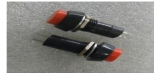
Gambar 2.10 Switch Push ON
